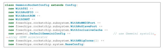
To build a simulation of this example Chipyard config, run the following commands:
