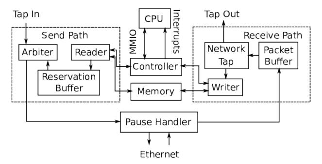
There are four basic parts of the NIC: the *Controller*, which takes requests from and sends responses to the CPU; the *Send Path*, which reads data from memory and sends it out to the network; the *Receive Path*, which receives data from the network and writes it to memory; and, optionally, the *Pause Handler*, which generates Ethernet pause frames for the purpose of flow control.
