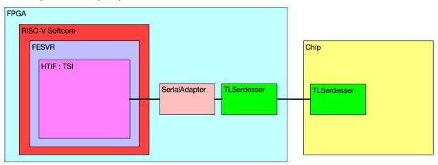
**Note:** The TLSerdesser can also be used as a slave (client), so it can sink memory requests from the chip and connect to off-chip backing memory. Or in other words, TLSerdesser creates a bi-directional TileLink interface.
