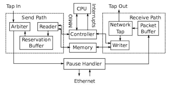
There are four basic parts of the NIC: the *Controller*, which takes requests from and sends responses to the CPU; the *Send Path*, which reads data from memory and sends it out to the network; the *Receive Path*, which receives data from the network and writes it to memory; and, optionally, the *Pause Handler*, which generates Ethernet pause frames for the purpose of flow control.
