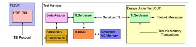
**Note:** Here the simulated AXI memory and the converters can be in a different clock domain in the test harness than the reference clock of the DUT. For example, the DUT can be clocked at 3.2GHz while the simulated AXI memory can be clocked at 1GHz. This functionality is done in the harness binder that instantiates the TSI collateral, TL-to-AXI converters, and simulated AXI memory. See *Creating Clocks in the Test Harness* on how to generate a clock in a harness binder.
