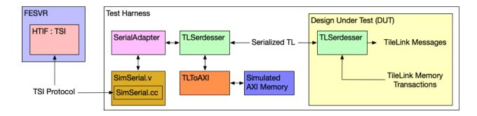
**Note:** Here the simulated AXI memory and the converters can be in a different clock domain in the test harness than the reference clock of the DUT. For example, the DUT can be clocked at 3.2GHz while the simulated AXI memory can be clocked at 1GHz. This functionality is done in the harness binder that instantiates the TSI collateral, TL-to-AXI converters, and simulated AXI memory. See *Creating Clocks in the Test Harness* on how to generate a clock in a harness binder.
