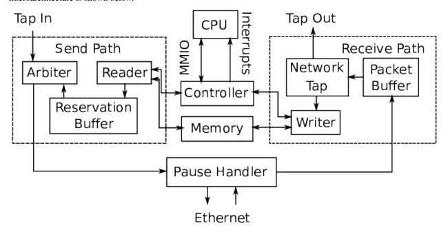
There are four basic parts of the NIC: the *Controller*, which takes requests from and sends responses to the CPU; the *Send Path*, which reads data from memory and sends it out to the network; the *Receive Path*, which receives data from the network and writes it to memory; and, optionally, the *Pause Handler*, which generates Ethernet pause frames for
