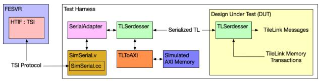
**Note:** Here the simulated AXI memory and the converters can be in a different clock domain in the test harness than the reference clock of the DUT. For example, the DUT can be clocked at 3.2GHz while the simulated AXI memory can be clocked at 1GHz. This functionality is done in the harness binder that instantiates the TSI collateral, TL-to-AXI converters, and simulated AXI memory. See *Creating Clocks in the Test Harness* on how to generate a clock in a harness binder.
